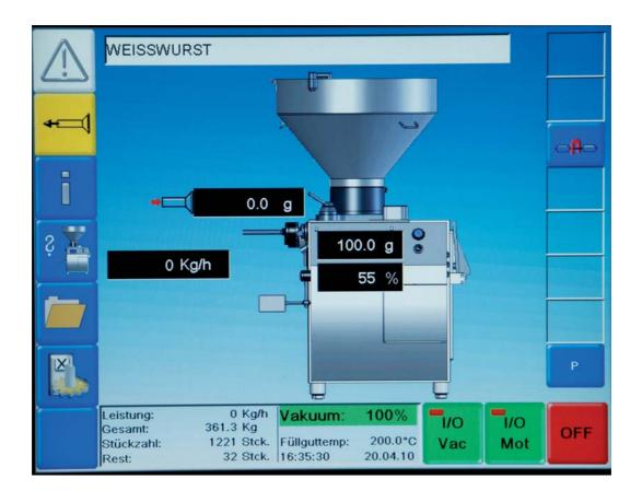
The ultimative stuffer control system with all variety of functions consists of an industrial personal computer and a touch screen panel in the front door of the filling machine.
